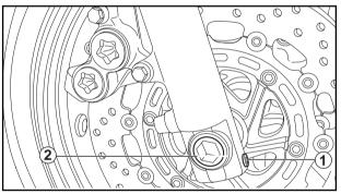
Brake disc bolt 25 Nm (2.5 m•kg) LOCTITE<sup>®</sup> 648
