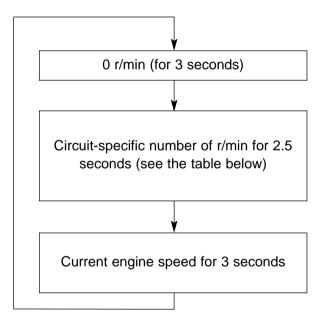
Use the chart below to identify the faulty electrical circuit.
