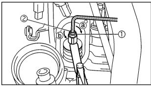
Measure the valve clearance with a thickness gauge (1).
