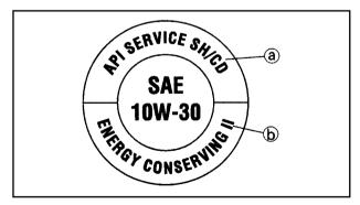
Recommended engine oil Refer to the chart for the engine oil grade which is best suited for certain atmospheric temperatures. API standard SE or higher grade ACEA standard G4 or G5
