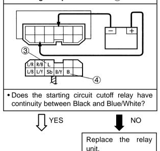
5. Starting circuit cutoff relay (diode)
