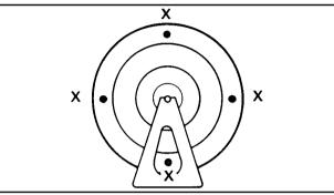
b. Turn the front wheel 90° so that the heavy spot is positioned as shown
