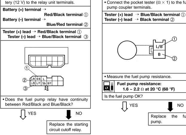
• Connect the pocket tester ( $\Omega \times 1$ ) and bat-
