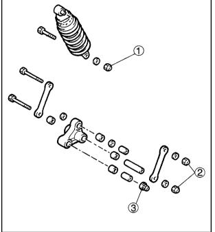
Rear-shock-absorber-assembly: Lower nut ① 50 Nm (5.0 m•kg) Connecting arm nuts ② 50 Nm (5.0 m•kg) Relay-arm-to-frame-nut ③ 50 Nm (5.0 m•kg)
