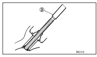
Out of specification  $\rightarrow$  Replace the valve guide.
